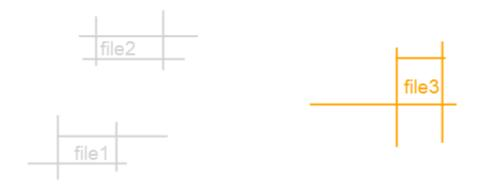
There is a shift of one drawing compared to the others. Originally all drawings had an identical coordinate system. Now the coordinate system of one drawing is shifted. This is not a change of the coordinates of individual objects, but a change of the position of the entire drawing.
